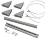
Use to mount CONCEPT, Networking and wall-mount enclosures to poles of various sizes and shapes. Simply attach the plated steel channel bar to the mounting holes at the back of the enclosure and wrap the stainless steel strap around the pole and through the bar. Kit includes two mounting channels, two straps suitable for 3-in. (76-mm) to 12-in. (305-mm) diameter pole and mounting hardware.
